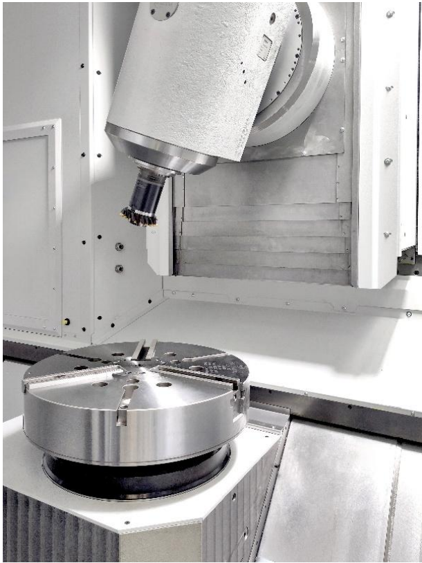
Image 5: The new HESSAPP VDM 750 Plus combines turning, gear skiving, and additional processes for precise and cost-effective complete machining of geared components.
