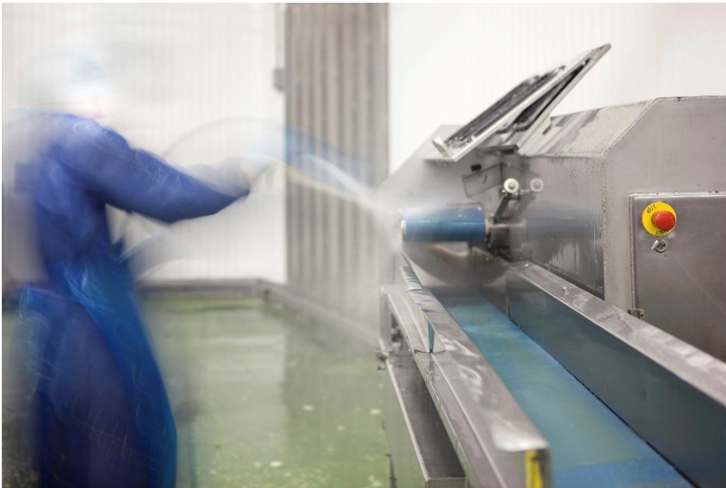
Image 1: Modern hygienic designs allow cleaning in place, reducing both contamination risk and downtime.
