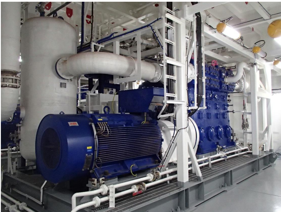
Image 2: A Burckhardt Compression Laby®-GI Compressor installed on an LNG carrier.
