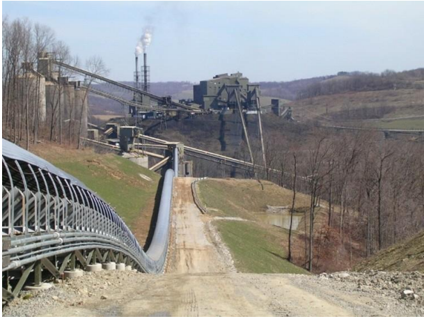
Image 3: Intelligent braking systems can improve the safety and durability of overland conveyors
