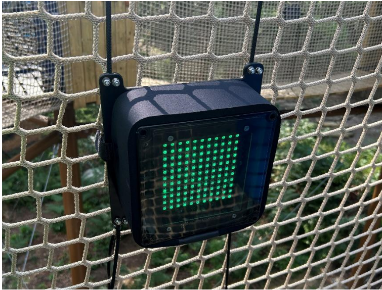
Image 3: Spelsberg TK Enclosure is water-resistant and capable of protecting the electronics from impacts.
