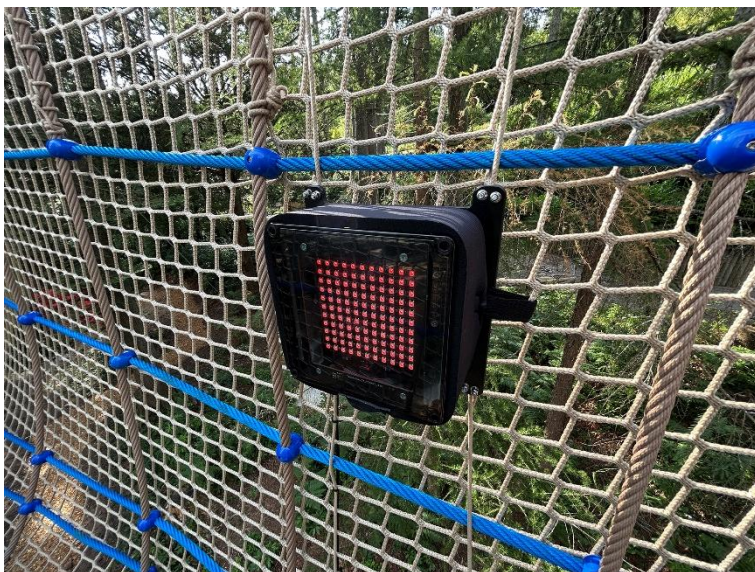
Image 4: Spelsberg TK Enclosure is water-resistant and capable of protecting the electronics from impacts.
