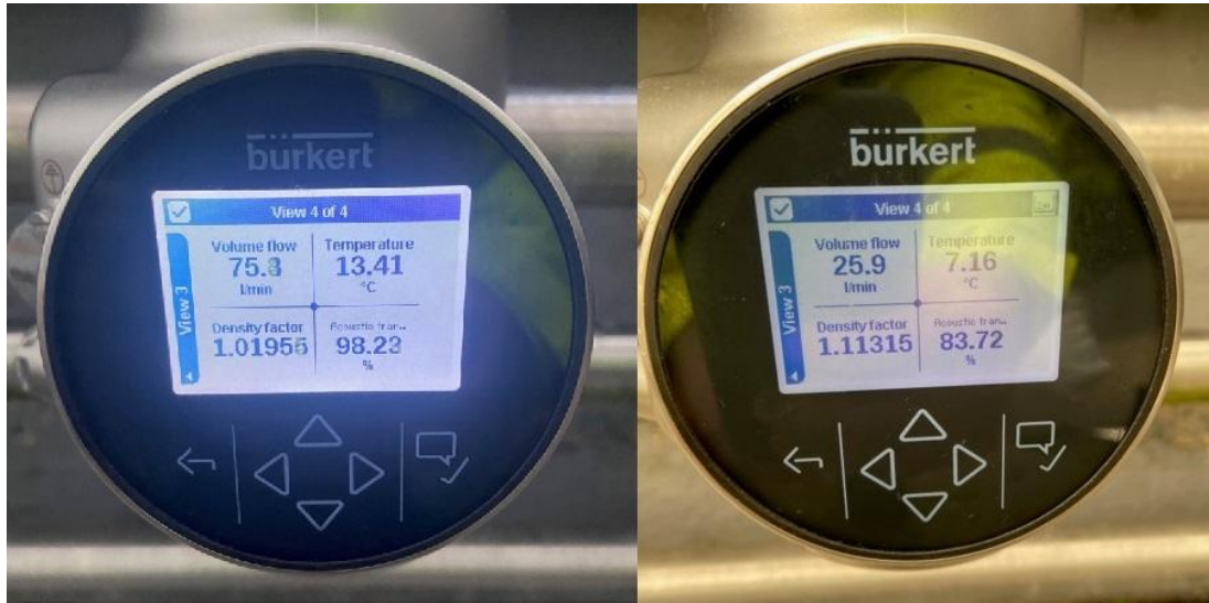
Image 3: FLOWave provides accurate measurements for different specifications of liquid whey.
