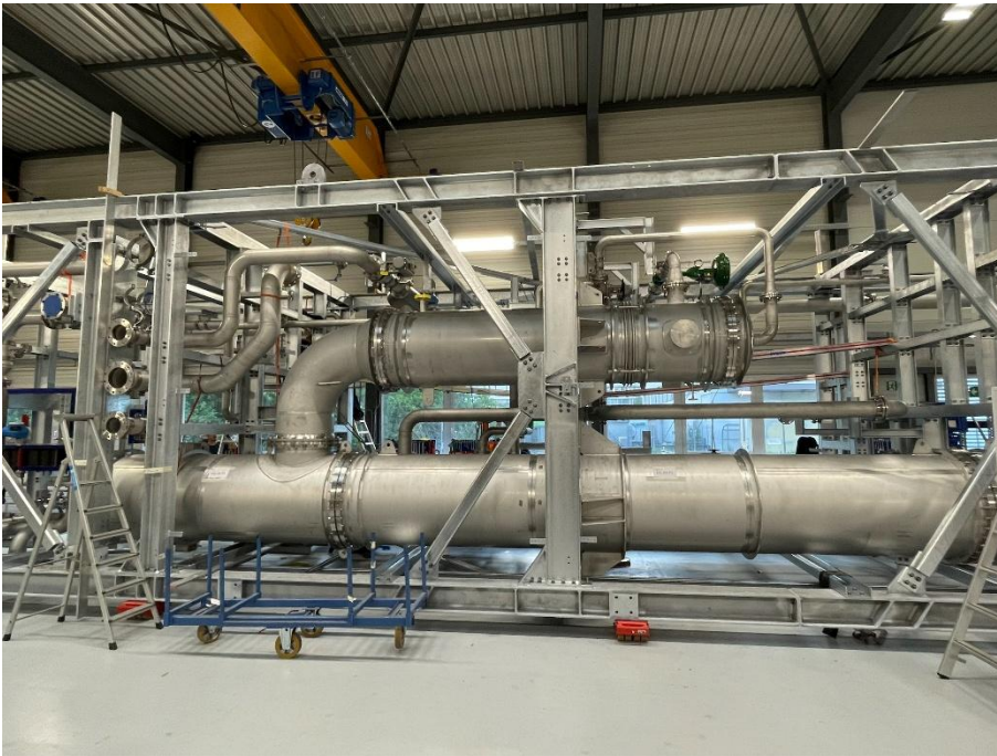
Image 1: EvapCare Unit Integrated with Distillation Column
