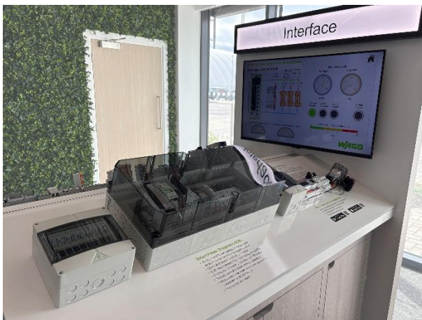
Image 2: Spelsberg specified a range of enclosures from its AK distribution board range for WAGO's demonstration unit.
