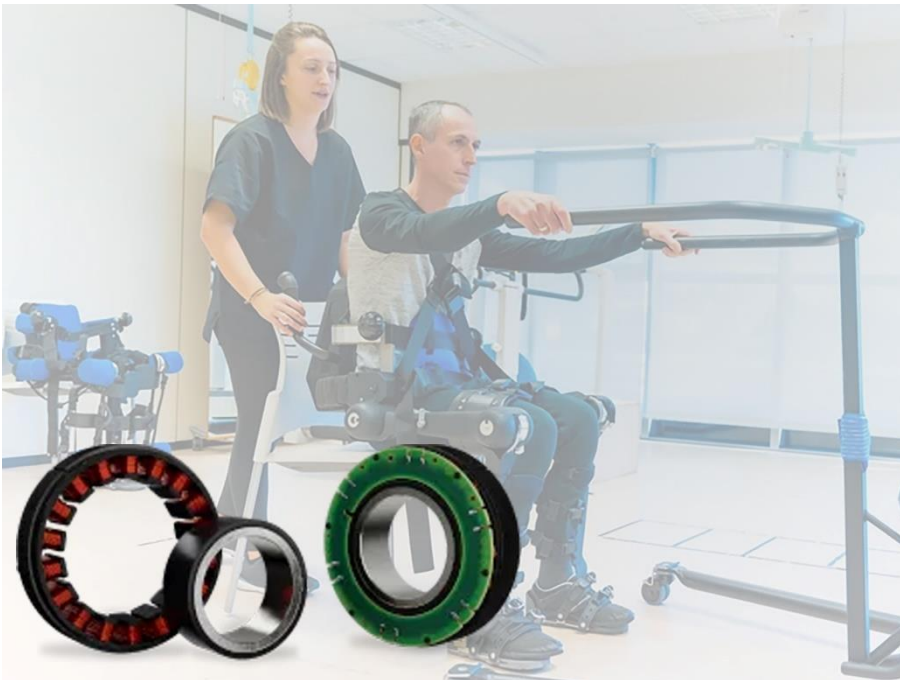
Image 1: Exoskeleton designers continue to see the advantages of frameless brushless DC (BLDC) motors such as the Kollmorgen TBM2G.
