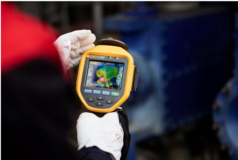
Image 5: Thermal anomalies can indicate potential problems like leakages, insufficient cooling, excessive friction or inadequate lubrication.
