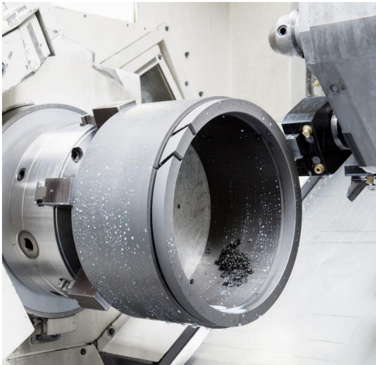
Image 2: Upgrade of rings & sealing elements with newest design.
