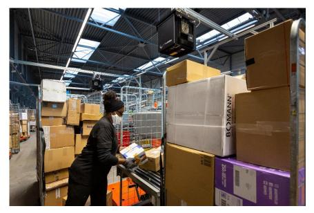
**Image 2:** Once a parcel has travelled through a sorting system, it ends up in a chute where workers will take the parcel, read the address label or scan the barcode, then place it in a cage ready for transfer to a buffer zone or loading area.
