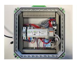
**Image 2:** WAGO has chosen the Spelsberg GTi series of polycarbonate distribution boxes as a convenient and aesthetic housing solution to house transportable demo systems.
