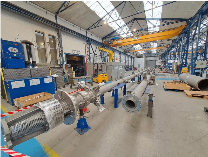
Image 2: The 2-stage, 35-meter-long SJS seawater lift pumps were delivered in record time
