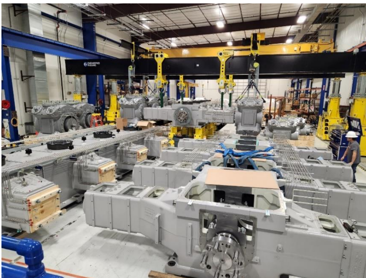
Image 4: Burckhardt Compression invested in a hydraulic gantry crane system with a 1-million-pound (450 ton) lifting capacity, which would allow the safe, slow movement of the compressors across the workshop.
