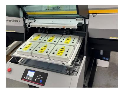
**Image 2: -** Printing logos and text directly on the Spelsberg Enclosures much more durable, especially when is used in an industrial or outdoor environment.
