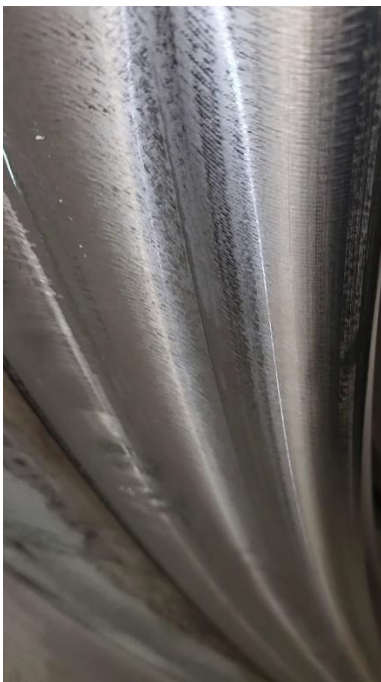
Image 4: Following resurfacing, yaw disc imperfections are removed, restoring braking performance.
