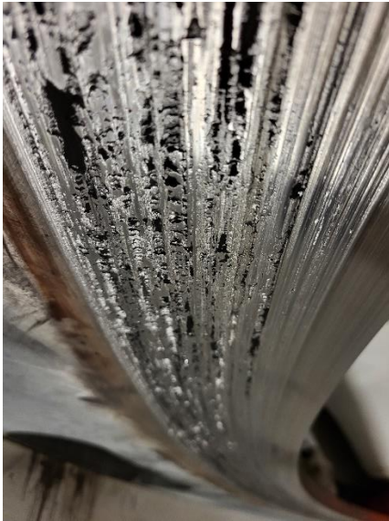
Image 3: A worn yaw disc before resurfacing.
