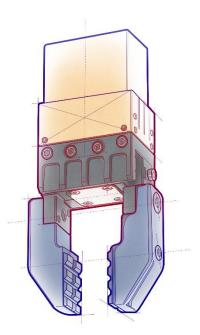
**Image 1:** Precise control of position, speed and torque can be achieved more effectively than with other types of actuation systems – making electric grippers ideal for complex manufacturing.
