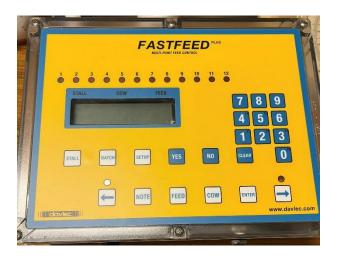
**Image 1:** Spelsberg industrial enclosure design, based on a lightweight, highstrength polycarbonate thermoplastic, provides protection against water and dust ingress, impacts and corrosion.
