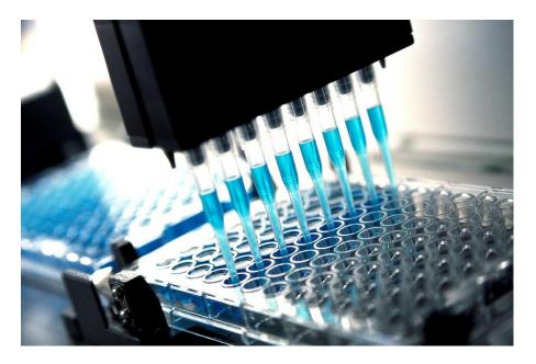
**Image 3:** Liquid handling workstations take on the repetitive tasks such as uncapping and recapping test tubes; dispensing liquid samples accurately; as well as mixing, stirring, and transporting processed test tubes.
