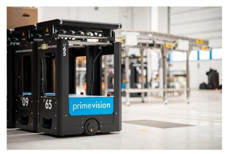
**Image 4:** By harnessing a computer vision system to check available capacity in each chute, robots can be directed to unload at a destination where room is available.
