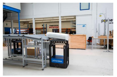
**Image 1:** Able to handle anything from a single letter to a 2-metre square parcel weighing well over 30 kg, robots can be equipped to move a wide range of items that would be totally unsuitable for a conveyor system.
