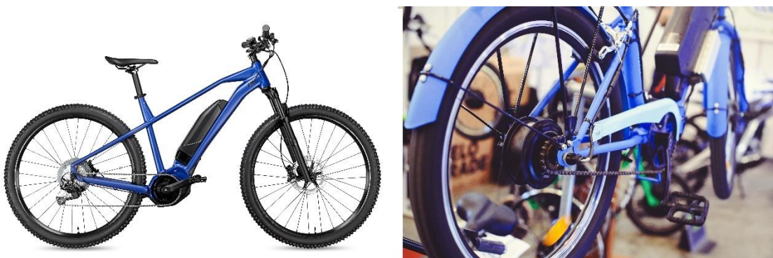
Figure 2: Mid-drive motor at center of bicycle (left); hub motor in rear wheel of bicycle (right)
