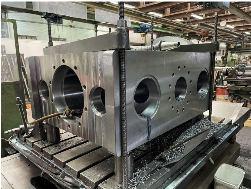
Image 2: Machining the new cylinder from a single forging.
