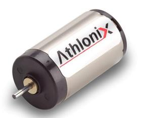
**Image 2:** When approached by a leading manufacturer of mechanical thrombectomy devices, Portescap selected its 16N78 brushed DC coreless motor, which can run efficiently at the high speeds required to achieve proper wire rotation and quickly break up a clot.
