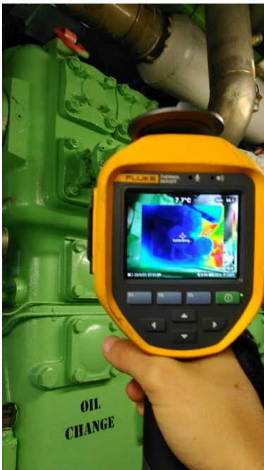
Image 4: Thermal imaging is one of the methods of identifying gas leakage, which can lead to reduced efficiency and reliability in a compressor. (for web use only)
