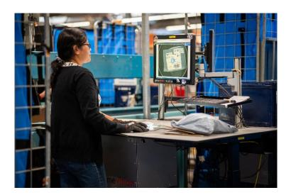
**Image 2:** A camera equipped with OCR technology can read each label, collecting individual parcel data and automatically transforming it into a pre-arrival submission, ready to be forwarded to postal services or customs.
