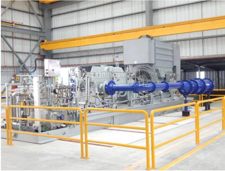
Image 1: The new state-of-the-art facility features a 10-meter-deep hydraulics test bed for large pumps, a digital monitoring system and a dedicated packaging area.
