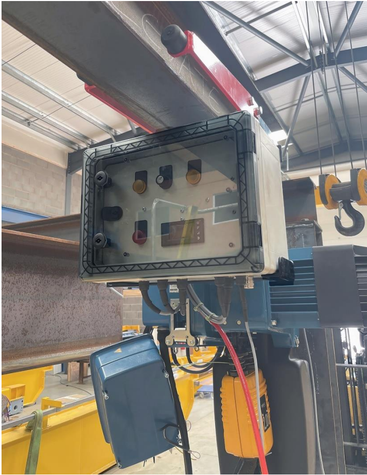
Image 1: Levate Solutions uses Spelsberg GEOS enclosure to protect crane control architecture from corrosion while enabling easy use for their own build process, as well as operator access.
