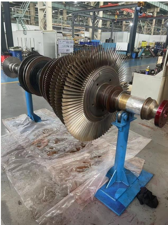
Image 4: Following reverse engineering, Sulzer manufactured new blades and re-bladed the turbine in-house, among other repairs.
