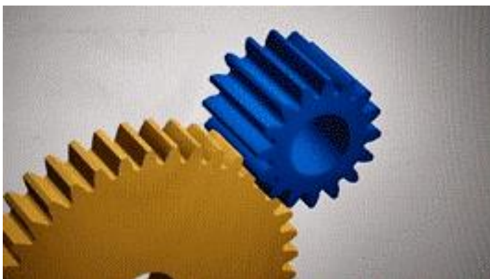
Image 2: Spur gears contact takes place simultaneously over the entire face width of the teeth, positioned in parallel to the gear's axis.
