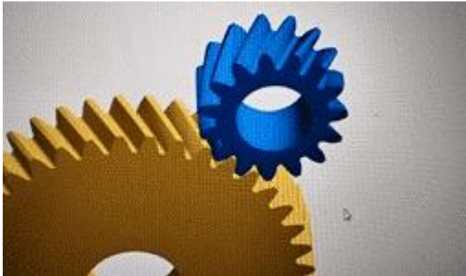
Image 1: The design of a helical gear ensures that the meshing teeth pair come into contact gradually and engage along a helical path.
