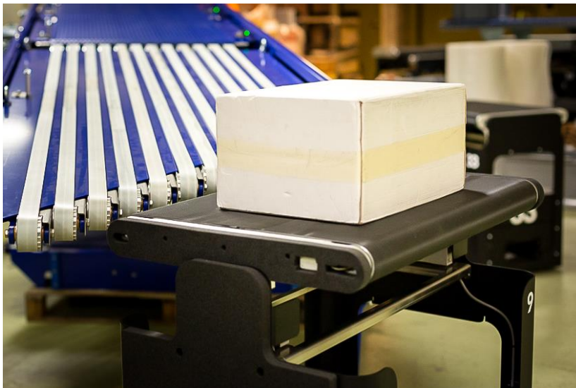
Image 2: With an 80 x 60 cm loading surface for parcels, Prime Vision robots offer a 35 kg carrying capacity.
