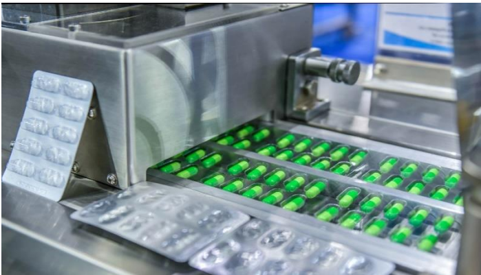
Image 2: Optimal Industrial Automation developed new blister pack inspection machines consisting of two vision systems to support a tablet manufacturer that was surprised by a sudden breakdown (Image source: iStock: 1285400923)
