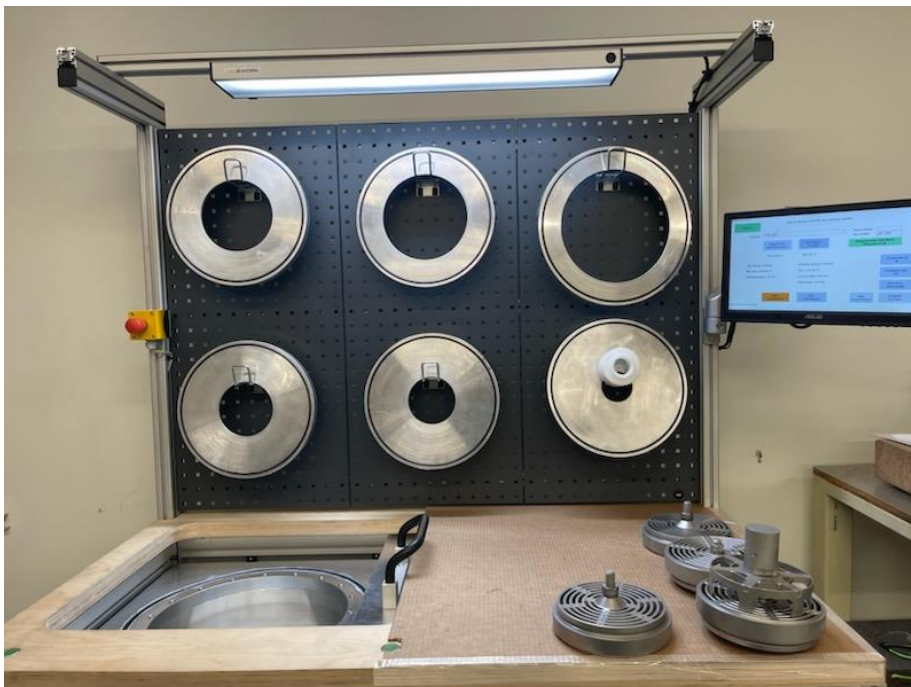
Image 2: The new testing station is fully equipped to handle numerous valve designs from any manufacturer.
