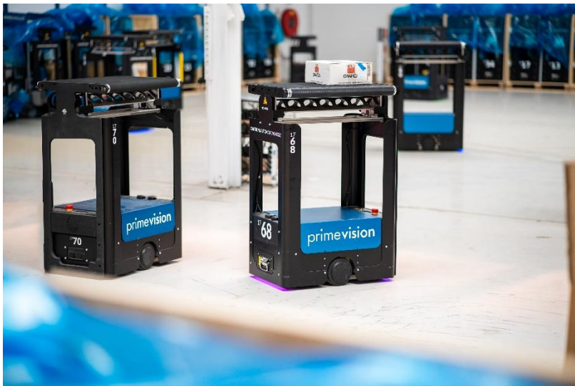
Image 2: Prime Vision robots navigate within a predefined area via a camera and sensors. If a robot spots an obstacle, it will stop automatically.
