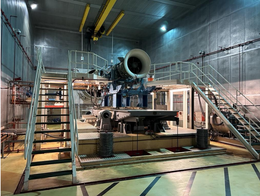
Image 1: An Avon Gas Turbine in the final phase of testing.
