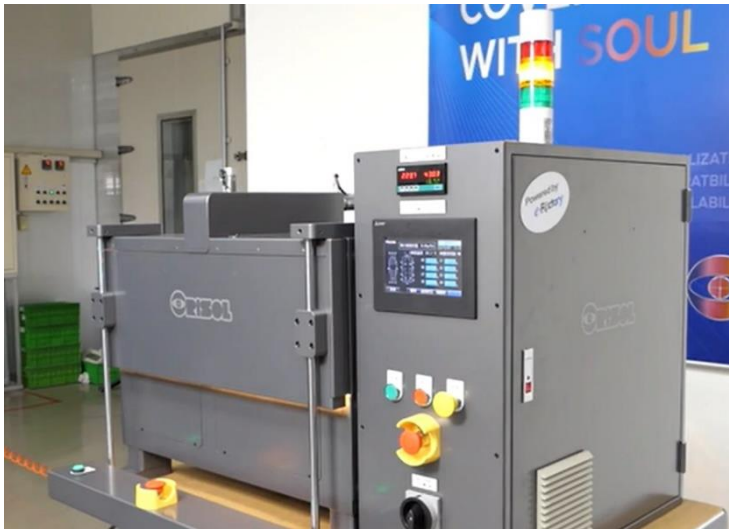
Image 3: Orisol saw its OFA240 series upper to sole flash activator machine as an ideal candidate to benefit from the principles of TSN technology. (© Orisol)
