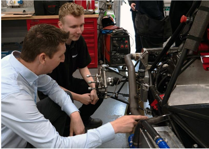
Image 1: Klarius manufactured a bespoke exhaust system for the Staffordshire University Formula Student race team
