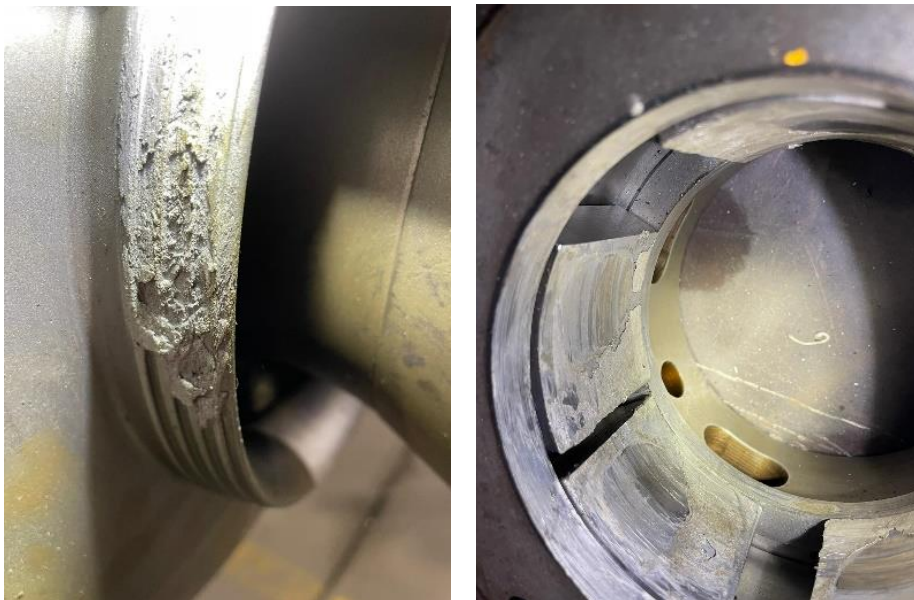
Image 2 + 3: It was suspected that the rotor was incorrectly aligned during installation, which led to the impellers making contact with the casing and causing damage to the seals.
