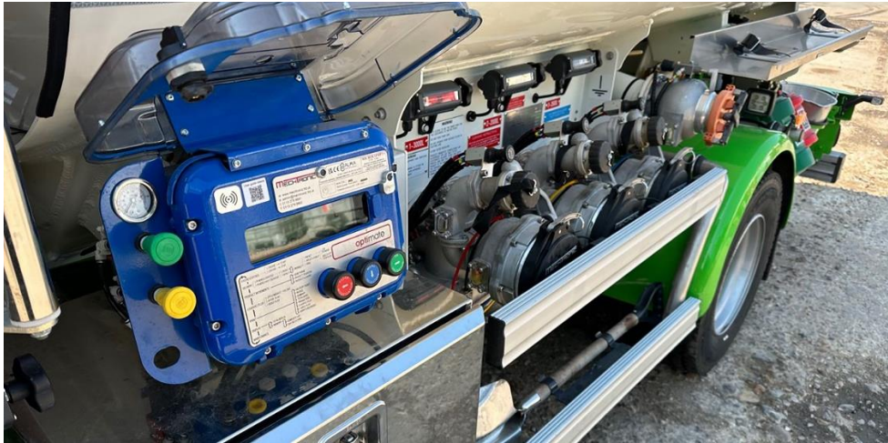
Image 1: MechTronic's truck-mounted fuel delivery systems comprise a variety of electronic components.
