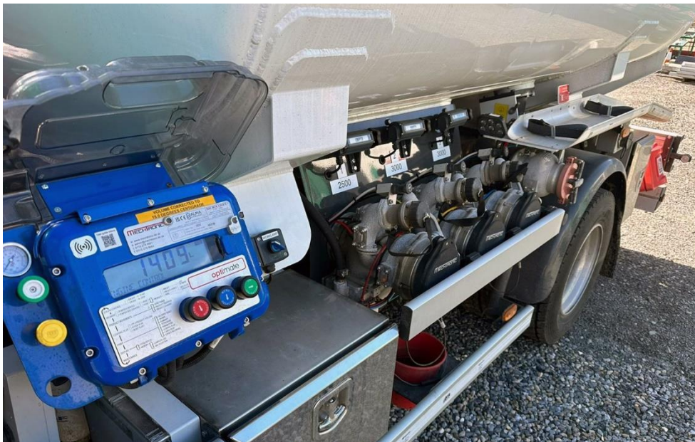
Image 2: MechTronic's truck-mounted fuel delivery systems comprise a variety of electronic components.
