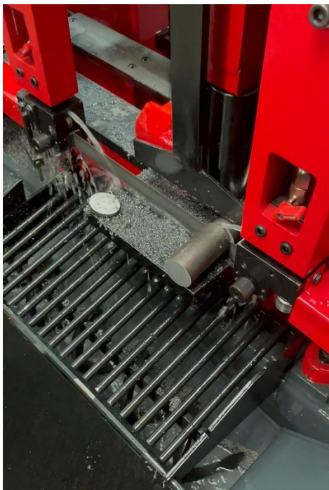
Image 2: The new band saw from WDS with programmable numerical control (NC), that guarantees meticulous precision in each cut and allows autonomous operation.
