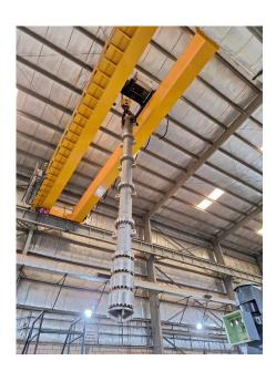
**Image 2:** Overhead cranes have been added to accommodate assembly, packaging and performance testing of some of the largest pumps in the Sulzer portfolio.
