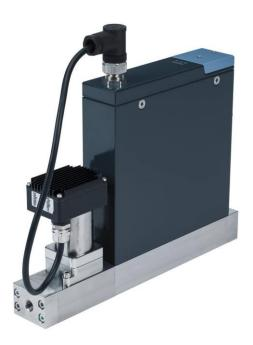
**Image 1:** Bürkert's Type 8756 mass flow meter/controller, based on the Coriolis effect, has a flow rate accuracy reading as low as  $\pm 0.2\%$ . This is achieved with a repeat accuracy deviation of just  $\pm 0.1\%$  for a flow rate up to 25 kg/h, or  $\pm 0.05\%$  repeatability for a flow rate up to 120 kg/h.
