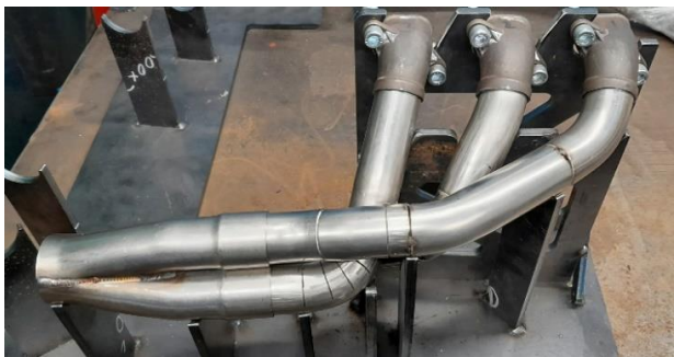
Image 2: KMT produced a bespoke welding jig to allow assembly of a custom racing exhaust for the Staffordshire Uni Racing team
