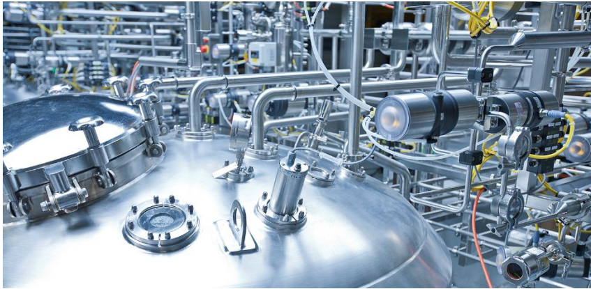
Image 1: The ideal solution is centred around a manifold that connects the tank directly to the process controller and control valves as well as the pressure sensor.
