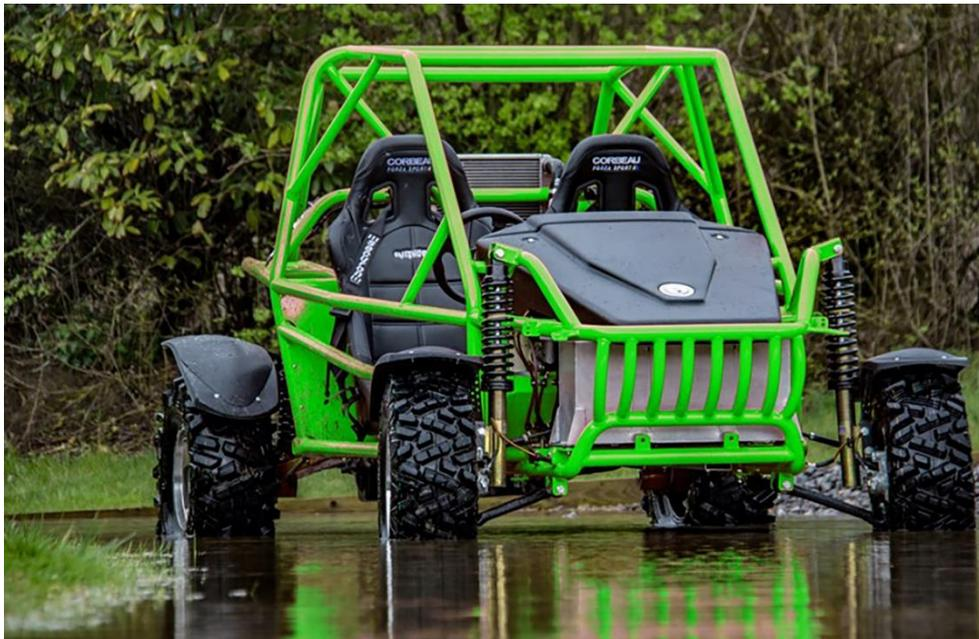
**Image 2:** Blitzworld buggy has Spelsberg enclosures, protecting the car's electrics and electronic control unit from the elements.
