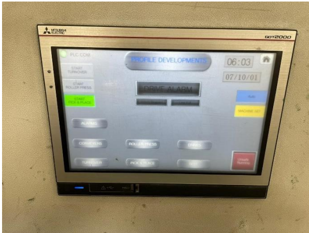
Image 3: An intuitive and user-friendly GT2510 widescreen HMI maximises process visibility and accessibility, helping operators monitor and interact with the drives, identify anomalies and interpret alarms. [Source: Mitsubishi Electric Ireland]
