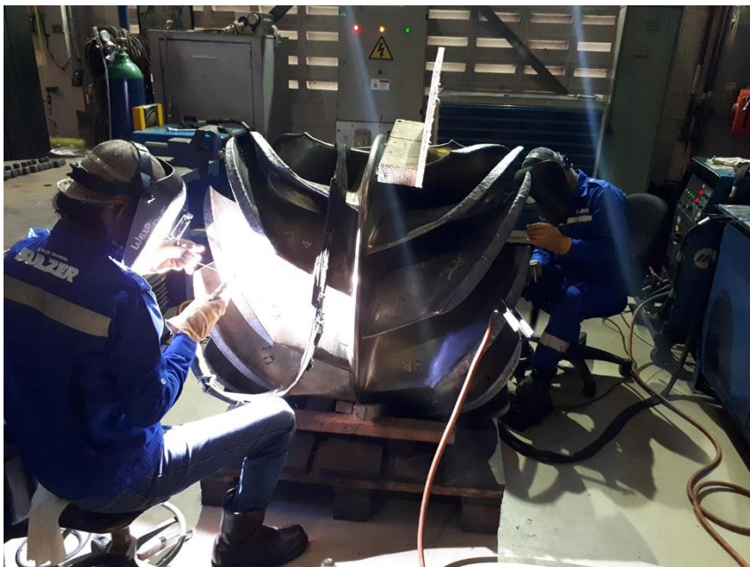
Image 2: Specialist welding processes were used to clad the blade tips with corrosion resistant material, ensuring an optimum repair.
