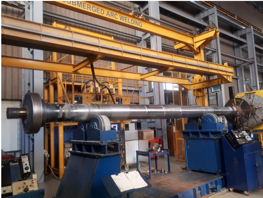
Image 1: Submerged arc welding (SAW) was used to apply an upgraded, high-strength low-alloy steel weld material, building up the diameter of the shaft.
