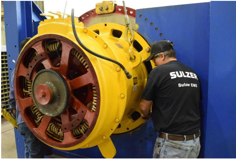
Image 1: Sulzer's in-house test rig for wheel motors ensures fast and effective overhauls
