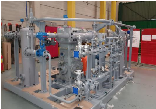
Image 2: Compressor skid during assembly.
