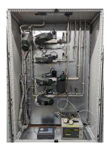
**Image 2:** In all three applications, the gas is controlled by a Type 8746 mass flow controller, while the nozzle gas is monitored by a Type 8742 mass flow monitor to ensure the correct nozzle pressure to deliver a droplet size between 30 and 120 microns.
